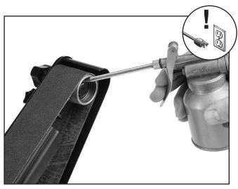
Figure 15. Lubricating the sleeve bearings.
